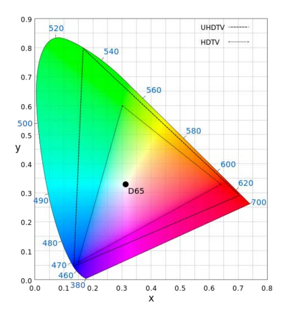
Diagram of the <u>CIE 1931 color space</u> that shows the <u>Rec. 2020</u> (UHDTV) <u>color space</u> in the outer triangle and <u>Rec. 709</u> (HDTV) color space in the inner triangle. Note that the Rec. 2020 came out in 2016 from the "UHD Alliance" an industry group, not from an international organization like the ITC nor a national one like SMPTE.
