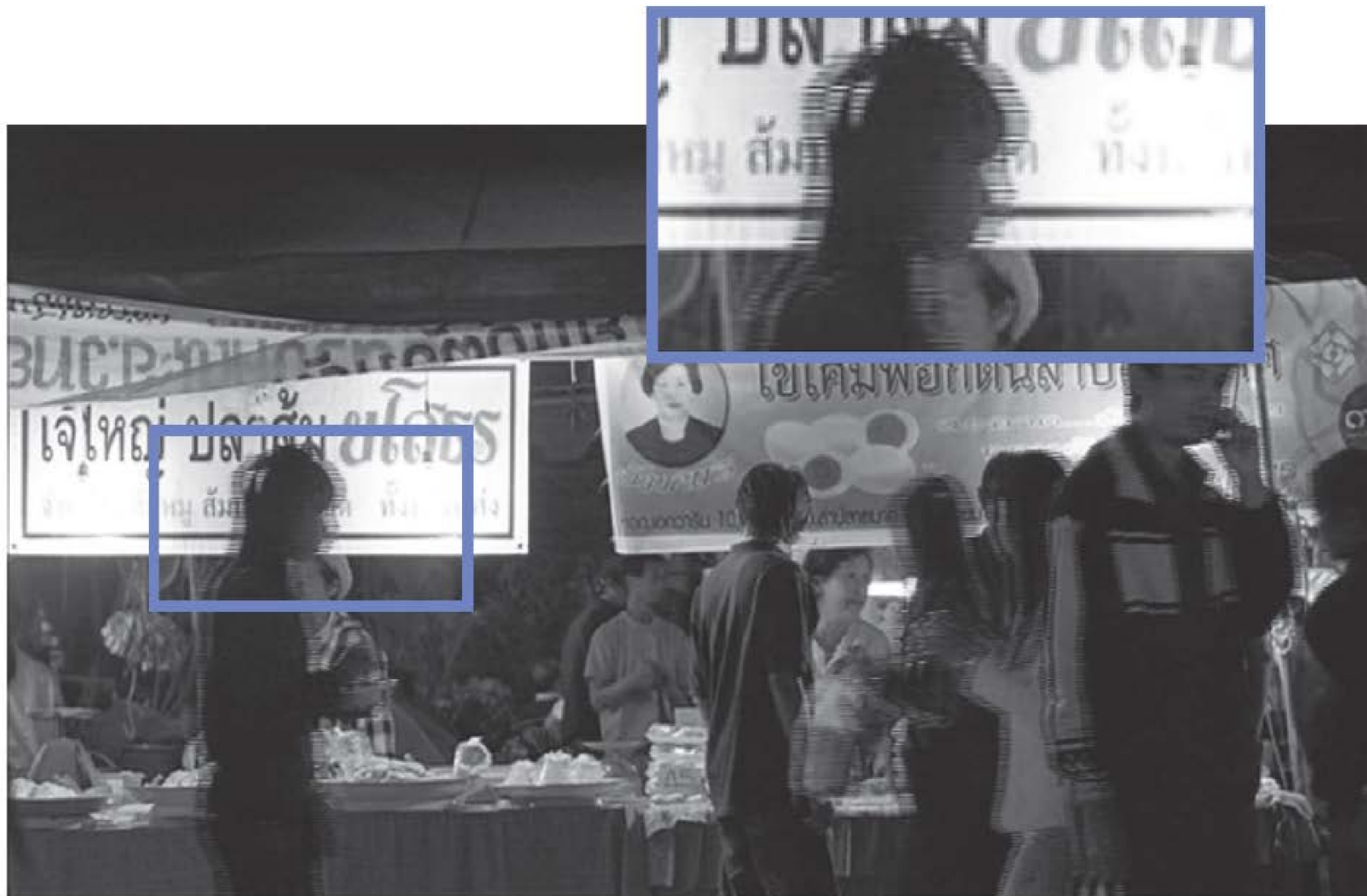
■ Figure 9-5 When interlaced video is shown on progressing displays, a “combing” artifact occurs at the edges of moving objects caused by the displaced scan lines (notice that the stationary objects do not show any combing).
